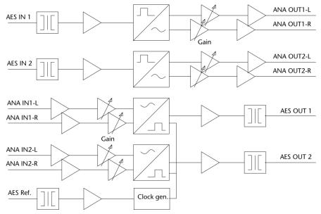
The ADDA-AES8 is an audio converter product with both A/D and D/A converters on a single module. The module may be used as a normal Flashlink module in the original frame, in N boxes and Flashcase. The module may also be used in the new frame in the half width slots as an auxiliary module for the Flashlink XMUX embedder modules.
