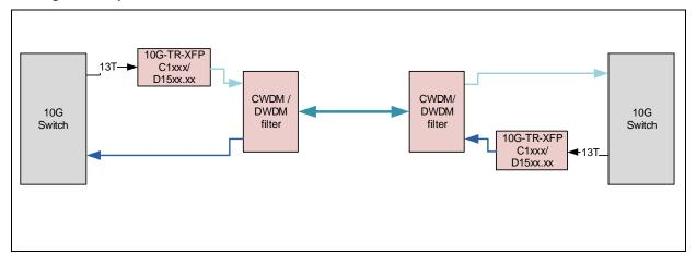
Figure 2: This figure shows a typical setup for wavelength conversion
