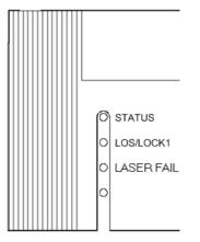
Figure 5: The 10G-TR has 3 LED's each showing a status.
